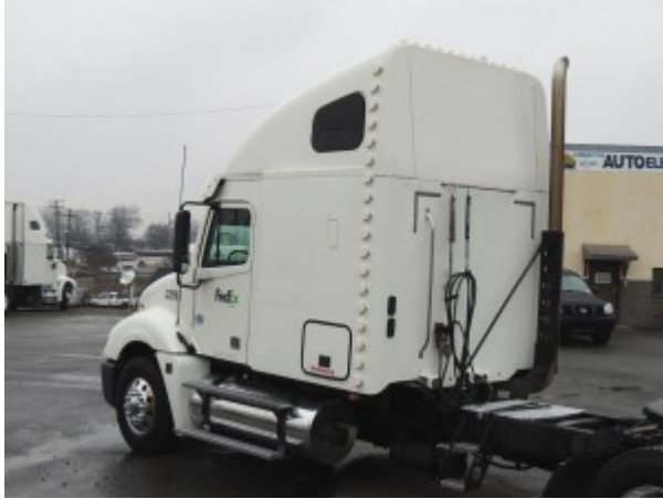
Figure 5. Vorblade tractor installation
