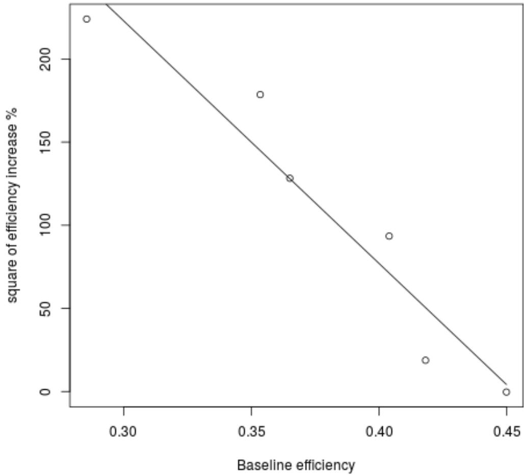
*Figure 6. Baseline efficiency vs. square of percent efficiency increase with least squares linear regression.*
