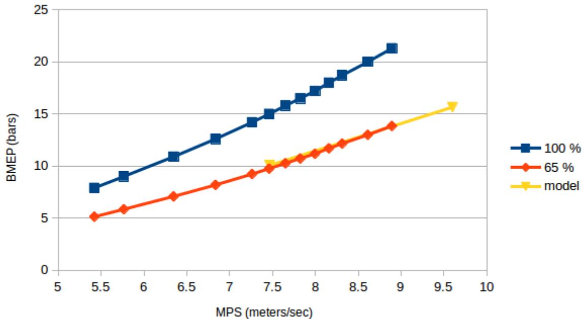
Figure 2. 100% and 60% load lines with model curve.
