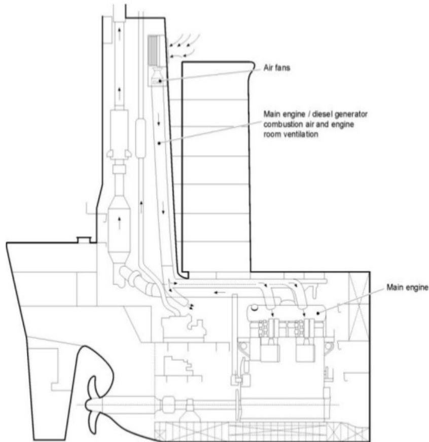
*Figure 1. Layout of Diesel propulsion system and electrical generators.*
